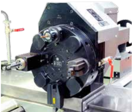
8-position with live tools (SE520)
